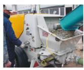
The Concrete Boy 350" can handle material up to a grain size of 16mm. With its integral automatic seal, it is even capable of pumping extremely low viscosity media with ease. The applications for which the fine concrete pump can be used range from spray concrete work to concrete pumping and the delivery of self-levelling screed and the pump fits a level into the gap between traditional worm pumps and heavy-duty pumps.
