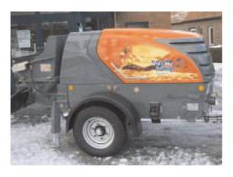
Spraying concrete, handling self-levelling screed, pumping concrete – the new compact concrete pump trailer is a veritable all-rounder. This small, lightweight and high-performance fine concrete pump is ideal for pumping anhydrite, cement and self-levelling cement screed, as well as fine cement and is perfect for spraying concrete, injecting mortar and all other concreting work up to a grain size of 32 mm.
