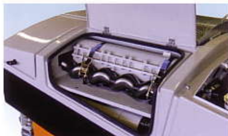
Storage compartment for replacement worm
