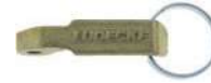
Handle with safety-ring and slotted pin made of malleable iron zinc-plated and yellow passivated (free of chrome VI)
