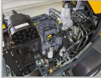
The robust, compact diesel engine meets all requirements of the "Stage V" emissions standard, applicable in the EU and Switzerland.
